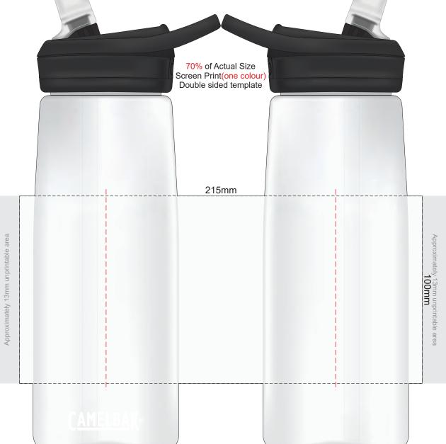
A 2-3mm tolerance is expected for alignment of the printed artwork and the CamelBak logo.
