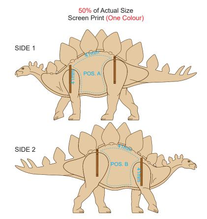
Up to a 2mm tolerance is expected for alignment of the printed artwork against the engraved lines. Slight inconsistencies are to be considered acceptable if the artwork is printed over an engraved line Blue Line = Safe area for Arwork
