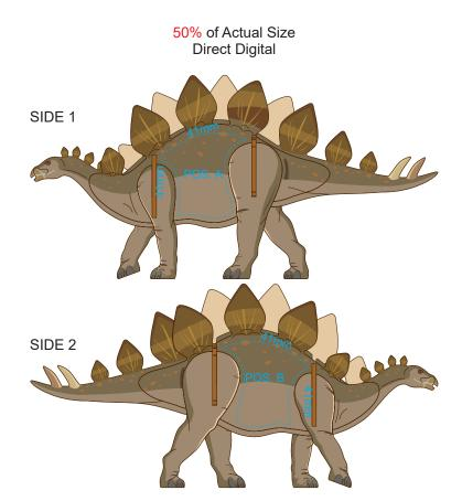
Up to a 2mm tolerance is expected for alignment of the printed artwork against the engraved lines. Slight inconsistencies are to be considered acceptable if the artwork is printed over an engraved line Blue Line = Safe area for Arwork
