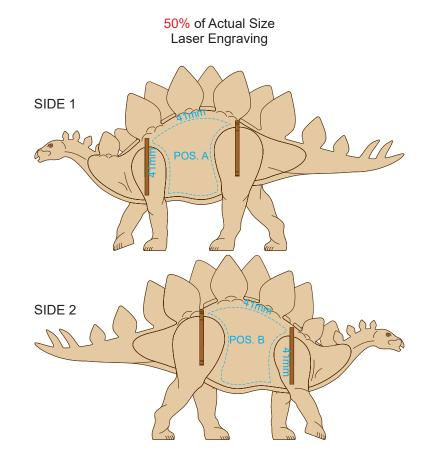
This product is a natural material, please allow for variances in grain pattern and engraving colour. Up to a 2mm tolerance is expected for alignment of the printed artwork against the engraved lines. Slight inconsistencies are to be considered acceptable if the artwork is printed over an engraved line Blue Line = Safe area for Arwork
